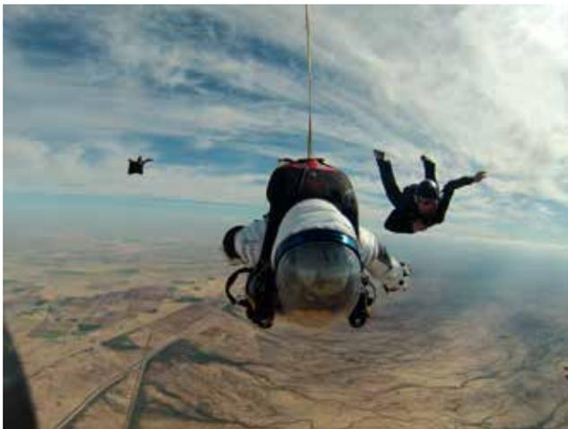
at altitude but also with the accumulation of carbon dioxide from the breathing apparatus. Dealing with the spin was an exercise in learning how to fall while wearing the suit. The result was the development of hand and arm movements that give control to the diver.
